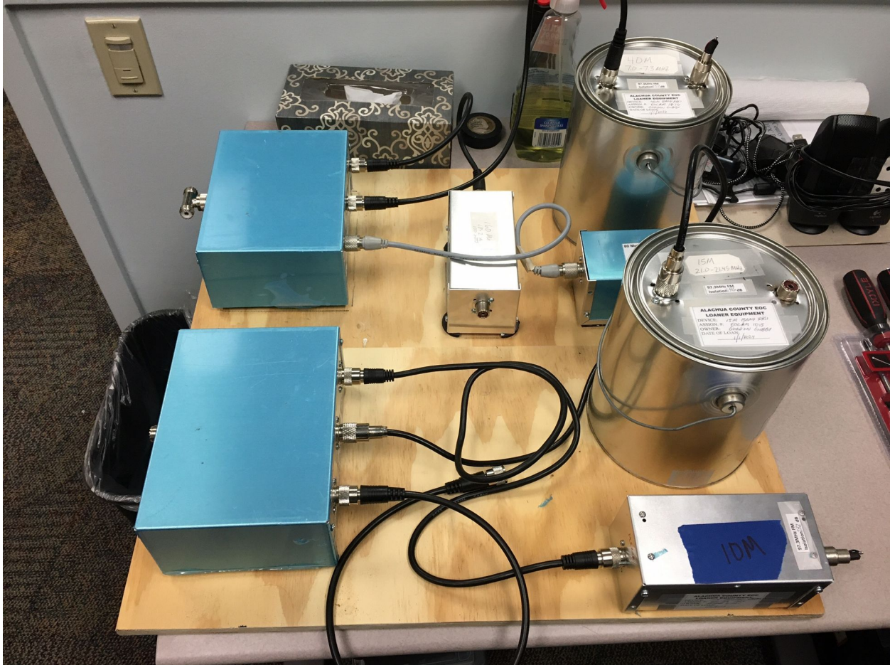
Mounting of Antenna Multiplexers and Filters
