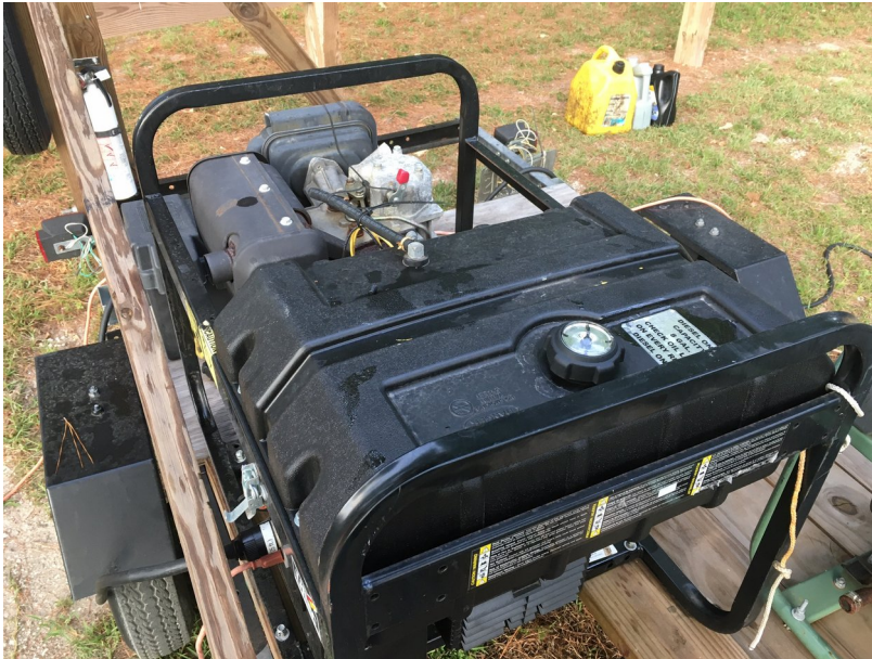
5kW Diesel generator Repaired and Refurbished for our group to use.
