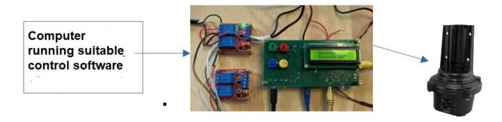
This allows low- or zero-cost satellite aiming software to be utilized with very inexpensive rotator systems -- even homebrewed rotators made from powerful linear actuators, and simple attached potentiometers for angular measurement So I decided to go that route instead of the "off-the-shelf" purchase route.
