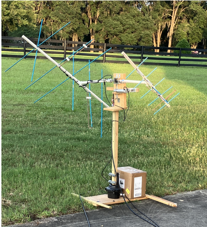
Figure: dual axis antenna rotator system with antennas
