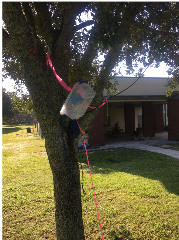
Safety isolation of the End Fed Half Wave Balun inside a plastic box hanging above head height on a tree.
