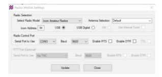
Note that "USB" rather than the USB-Digital is selected -- this allows the external PACTOR modem to send and receive signals via the analog cable to the rear panel ACCESSORY connection.
