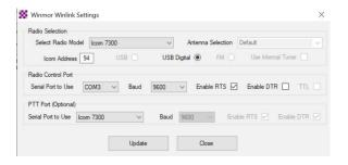
(ARDOP is similar) **Note that USB Digital is selected**. This allows the computer to control to send and receive via the USB (universal serial bus) connection.
