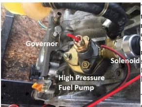
TIMING: Shims are available from several suppliers; the Ebay supplier had most understanding ordering mechanism. Multiple 0.1mm, 0.2mm and 0.3mm shims ordered; each 0.1 mm gives approx 1 degree of delay. The tappets were also different -- the older tappet gave more delay. When the shims arrived, I assembled my setup, got the solenoid open, made tedious measurements for multiple tries and over an hour and finally settled that I was "close" to the proper timing.
