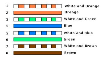
REF: <u>http://pinouts.ru/NetworkCables/Ethernet10BaseTStraightThru\_pinout.shtml</u> Reproduced by permission (presentation of http:// reference) To take advantage of the noise-reduction provided by the twisted pairs, I recommend using the following colors and settings:
