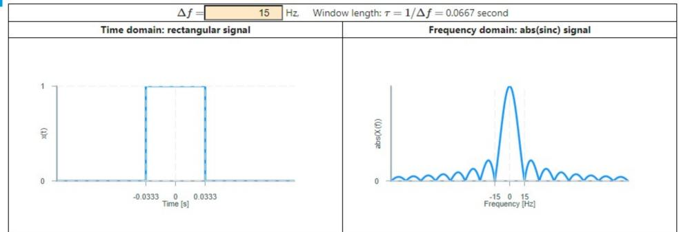
On a single "subcarrier" audio tone, sending that audio tone for a small slice of time [symbol rate] (a rectangle in the time domain) causes it to have "sidelobes" that look like the right hand graph – a sinx/x type (sinc) function. That subcarrier has a strong point, and many NULLS. We position the surrounding audio frequency subcarriers cleverly at the NULLS of their brethren.
